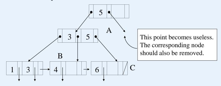
For this merge, 5 will be taken as a key value in A since any key value in B is less than or equal to 5 but any key value in C is larger than 5.
