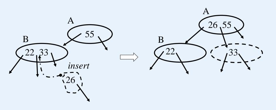
Note that '26' does not remain in B. This is different from the leaf node splitting.
