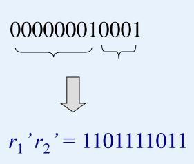
Starting at the beginning, find the first 0 at the  $3^{rd}$  bit, so j = 3. The next 3 bits are 111, so we determine that the first integer is 7. In the same way, we can decode 1011.
