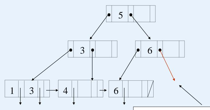
Deleting 7 makes this pointer no use. Therefore, a merge at the level above the leaf level occurs.
